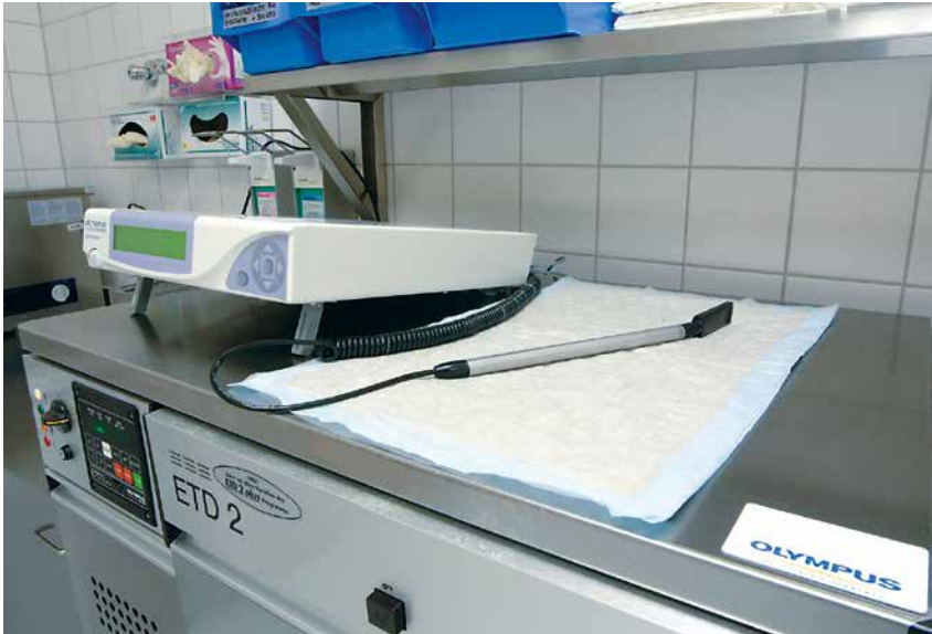
Figure 3: There are also big changes in the operating elements. The comparison shows the programming of an ETD2 in 2001 with a supplemental module for documentation using a hand scanner...
