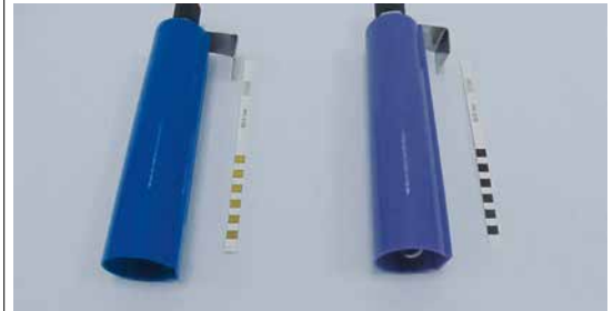
Cycle in accordance to annex B.2 "Fail" cycle – modified air removal stage
