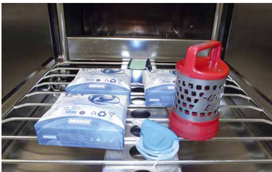
Fig. 3b: Arrangement of Browne, Melacontrol and EBI16 in the chamber for the test
